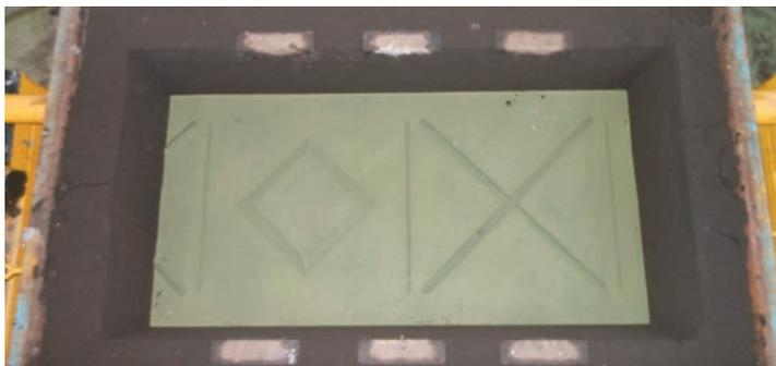
The main difficulty resided in defining the dimensions of the panels taking into consideration the deformation of the metal caused by stamping, and at the same time ensuring the system remains watertight. And subsequently in creating the stamping and bending die to test the quality of the product.
